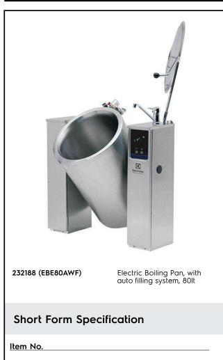
Stainless steel construction with the deep drawn pan with rounded edges manufactured from AISI 304 stainless steel. Pan can be tilted beyond 90° to completely empty the food. Motorised tilting with tilting axis located in the middle of the pan to keep the pouring lip high and allow tall vessels to be filled. Automatic water filling of the steam generator.
